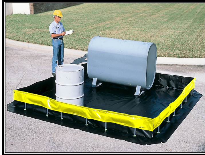
Figure IV - 5.6 Temporary Spill Containment.
