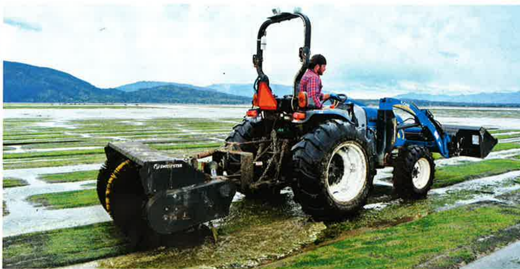
Attaching a standard city street sweeper to a New Holland Boomer™ compact tractor helps remove thick growth of algae that accumulates on plastic netting protecting growing clams.
