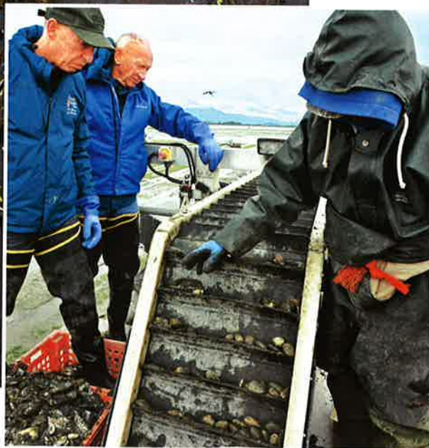
Bill Taylor (in front) and his brother Paul Taylor check on how clams are rotating through a modified tulip bulb digger and conveyor belt.
