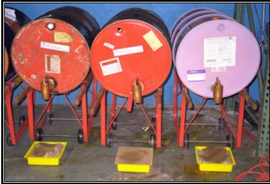
Figure 4.18. Mounted Containers with Drip Pans.
