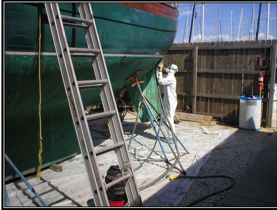
Figure 4.22. Drop Cloth Used During Hull Sanding.
