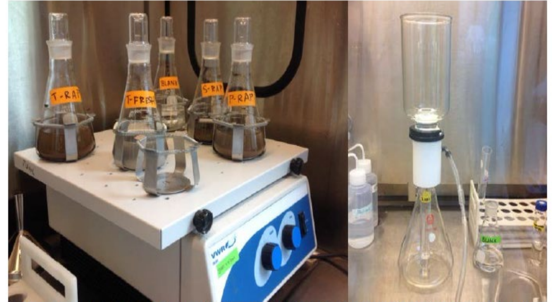
Figure 11: Laboratory Setup for Batch Extraction Experiments.
