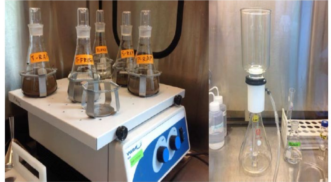
Figure 11: Laboratory Setup for Batch Extraction Experiments.
