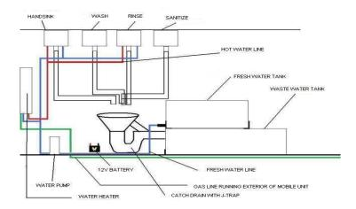
[EXAMPLE: PLUMBING SCHEMATIC (note air gap between sinks and waste tank)]
