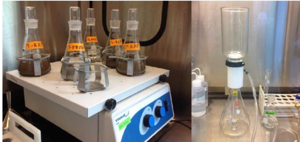
Figure 11: Laboratory Setup for Batch Extraction Experiments.
