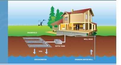
Many households in Thurston County depend on on-site septic systems to treat and dispose of sewage and wastewater from their homes. A well designed, installed, and maintained septic system can provide years of reliable service. **Regular maintenance is the key!**
