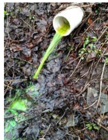
Dye Identified in Run Off Pipe. Please note: most failures are not so obvious.
