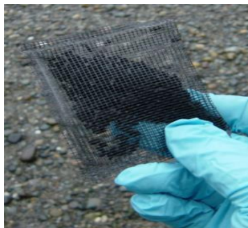
Charcoal Packet Used for Dye Test
