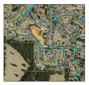
**Description:** The project will retrofit the existing Meadows Subdivision Pond 4C by regrading the site and replacing inlet and outlet structures to meet current water quality treatment and flow control standards. **Location:** Meadows Subdivision between Clover Loop SE and Gadwell Ct. SE between Steilacoom Rd. SE and Pacific Hwy SE.
