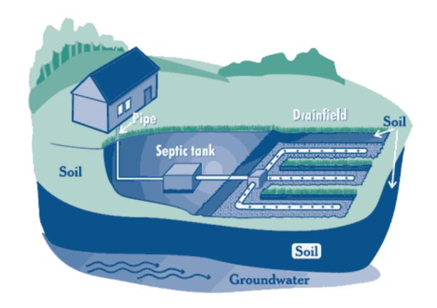
Simple; No mechanical parts; Soil does treatment; No OPC
