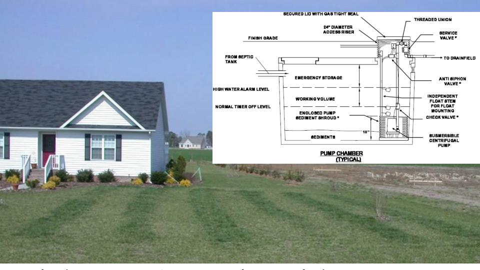
Includes pump & controls; Soil does treatment; No OPC
