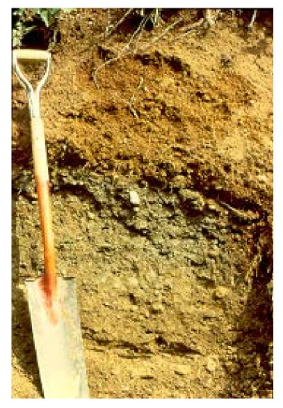
Shallow topsoil over very dense Glacial till provides minimal treatment and disposal.
