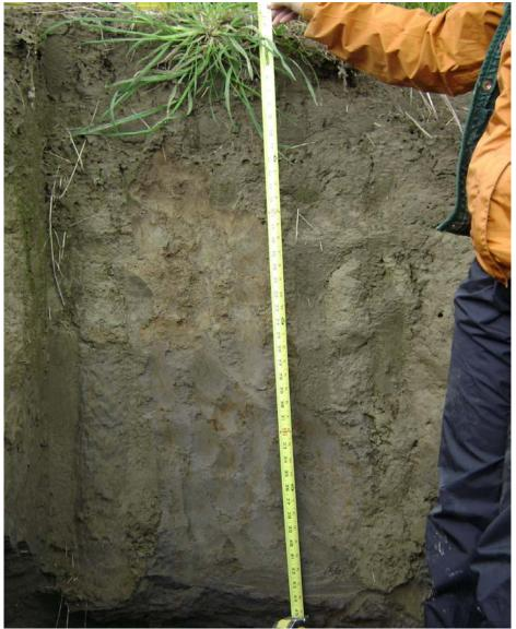
Drainage - Soil colors can mean a slow permeability or a high water table. Saturated soils provide poor disposal and treatment
