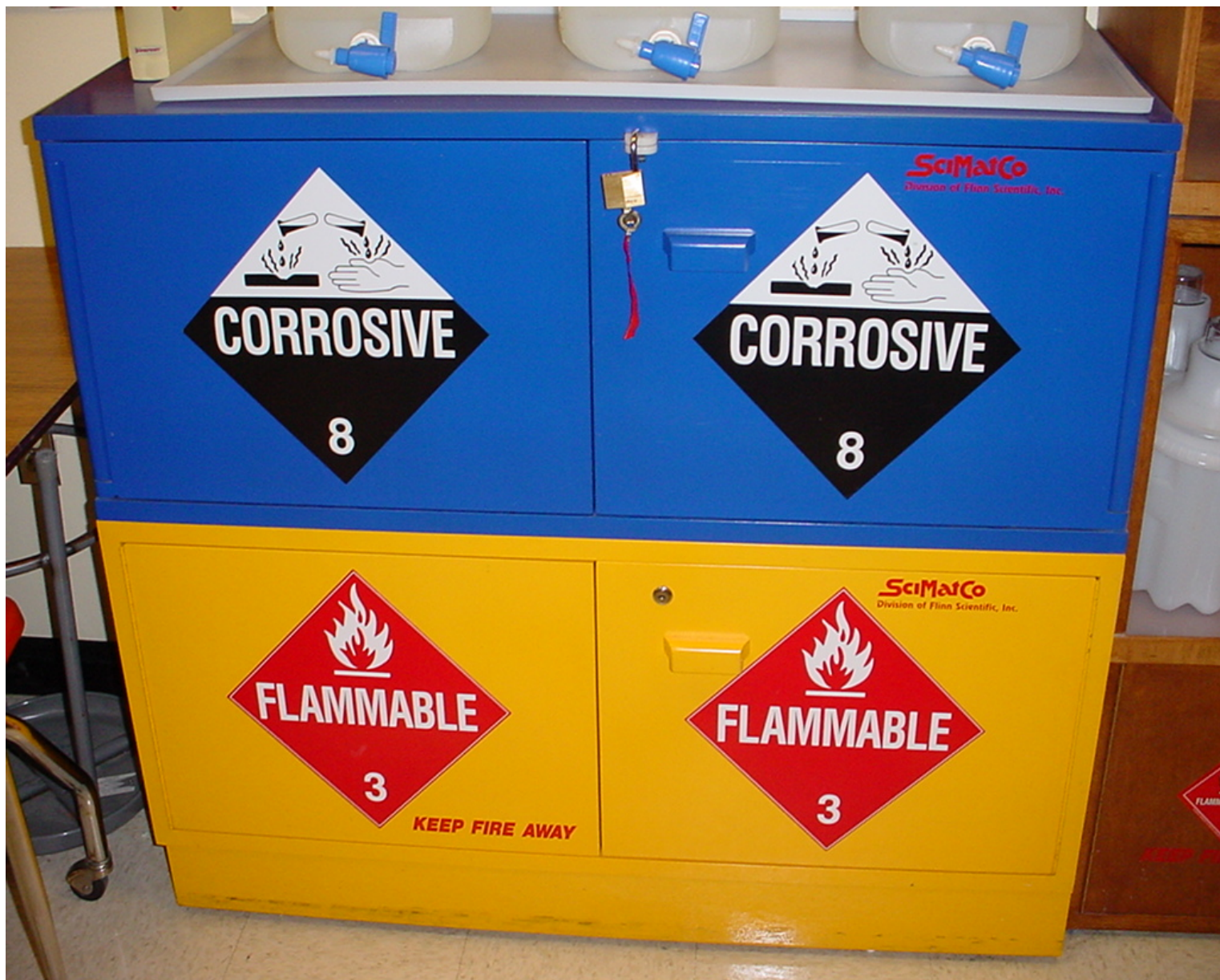
The Good: Example of proper storage cabinets and labeling.
