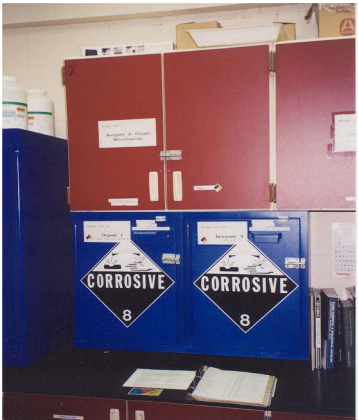
The Good: Appropriate storage cabinets with earthquake latches.
