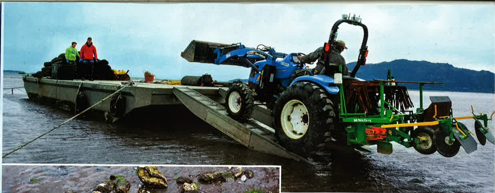
Taylor Shellfish Farms keep its New Holland Boomer™ tractor on a floating platform at its south Puget Sound location, Samish Bay. It's used when the tide goes out and the rows of growing clams are exposed. The attachment on the back is a Rain-Flo flat bed mulch layer.
