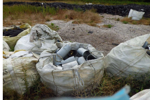
Stored Geoduck gear in the open at Kennedy Creek Natural Area Preserve, 2023. PVC foreground shows breakage, HDPE mesh “sleeves” in piles at the back. All are in the open, exposed to UV light.
