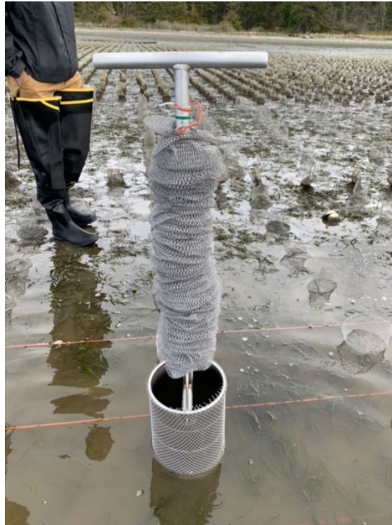
Photo 5. Modified clam gun used to install VEXAR mesh tube.
