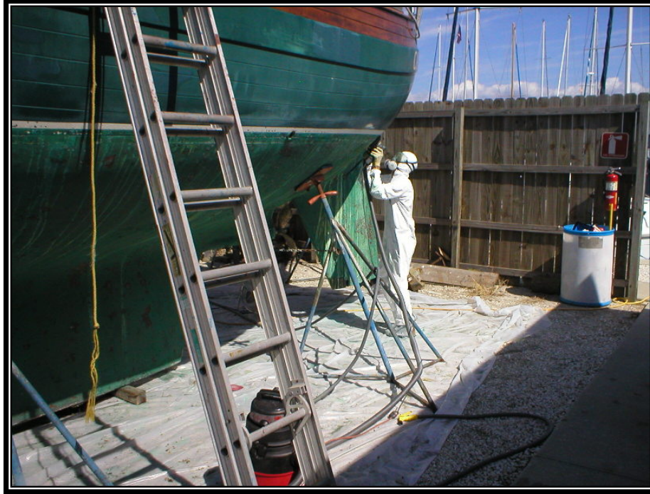
Figure 4.22. Drop Cloth Used During Hull Sanding.
