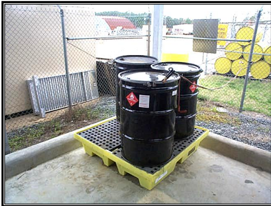
Figure 4.17. Temporary Secondary Containment.
