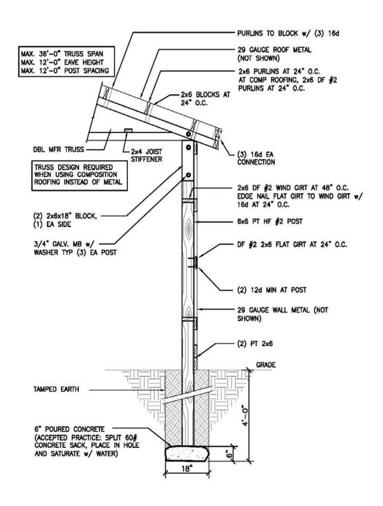
Pressure treated wood complying with AWPA U1 is required.
