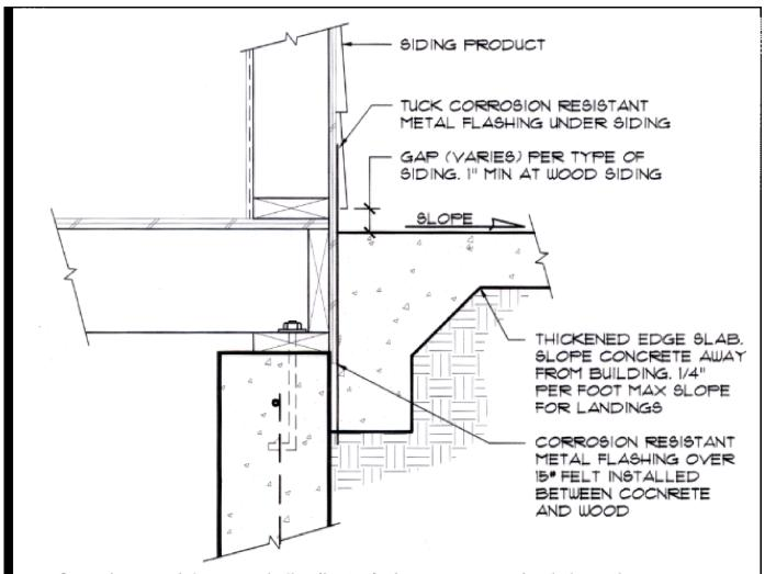
Concrete cannot be poured directly against non-pressure treated wood nor can concrete be poured against manufactured siding.
