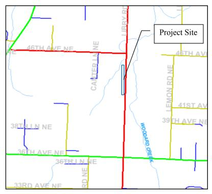
**DESCRIPTION:** Install an enhanced ditch, compost amended biofiltration swale or a bioretention swale and a filter vault within the Thurston County road Right-of-Way. This project was one of 5 projects identified in the 2014 Woodard Retrofit Study.
