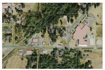
**Description:** Install approximately 1,100 feet of biofiltration swales and bioretention areas around Littlerock Elementary School, 127 Ave SW, and 128th Ave SW to improve water quality before discharging to the Black River and Beaver Creek Location: Along Littlerock Road SW, 127 Ave SW, and 128th Ave SW in the vicinity
