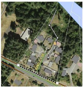
**Description:** Shorten outfall pipe and install an infiltration trench to provide water quality treatment and flow control before discharging into Deschutes River.
