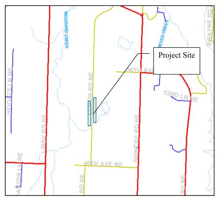
**DESCRIPTION:** Install enhanced ditches and a filter vault within the Thurston County road Right-of-Way, before discharging to a tributary of Woodard Creek. This project was one of 5 projects identified in the 2014 Woodard Retrofit Study.
