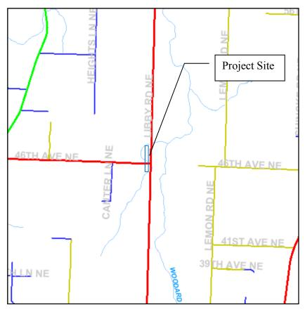
**DESCRIPTION:** Install bioretention cells within the Thurston County road right-of-way to filter the water before discharging to a tributary of Woodard Creek. This project was one of 5 projects identified in the 2014 Woodard Retrofit Study.
