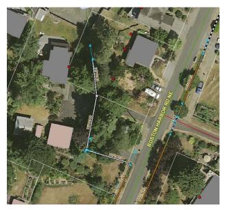
**Description:** Repair/replace failing outfall on Boston Harbor Road and add a culvert under Boston Harbor Road to reduce flooding.
