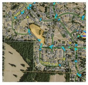
**Description:** The project will retrofit the existing Meadows Subdivision Pond 4C by regrading the site and replacing inlet and outlet structures to meet current water quality treatment and flow control standards.
