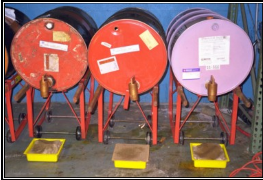
Figure 4.18. Mounted Containers with Drip Pans.
