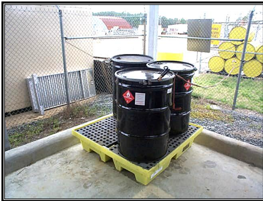
Figure 4.17. Temporary Secondary Containment.
