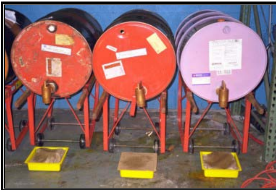
Figure 4.18. Mounted Containers with Drip Pans.
