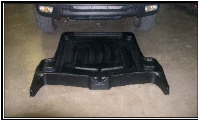
Figure 4.8. Drip Pan for Use at Mobile Sites.
