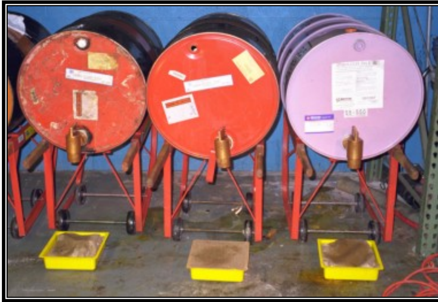
Figure 4.18. Mounted Containers with Drip Pans.
