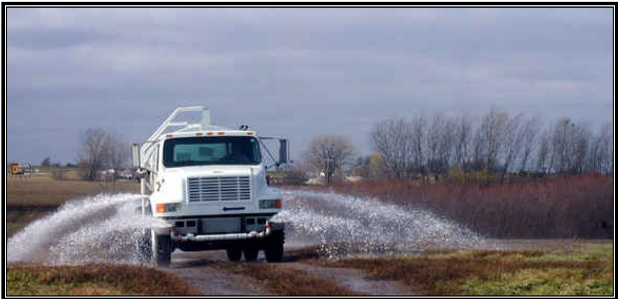
Figure IV - 4.21 Dust Suppression by Water Spray.
