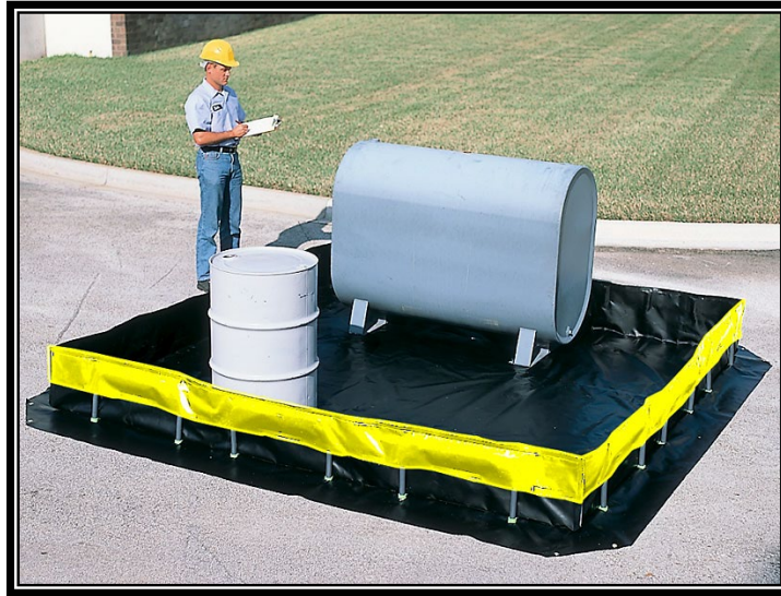
Figure IV - 5.6 Temporary Spill Containment.
