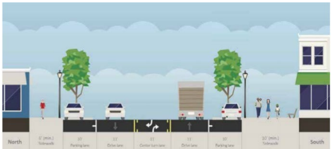
Figure 2. Conceptual design of Phase 1 – US 12 Cross-section Source: Main Street Rochester Multimodal Transportation Plan, 2019
