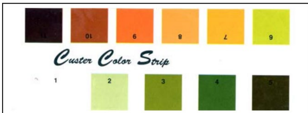
Figure 2. TCEH compared the color of the water on the Secchi disk (1 m) to the Custer Color Strip
