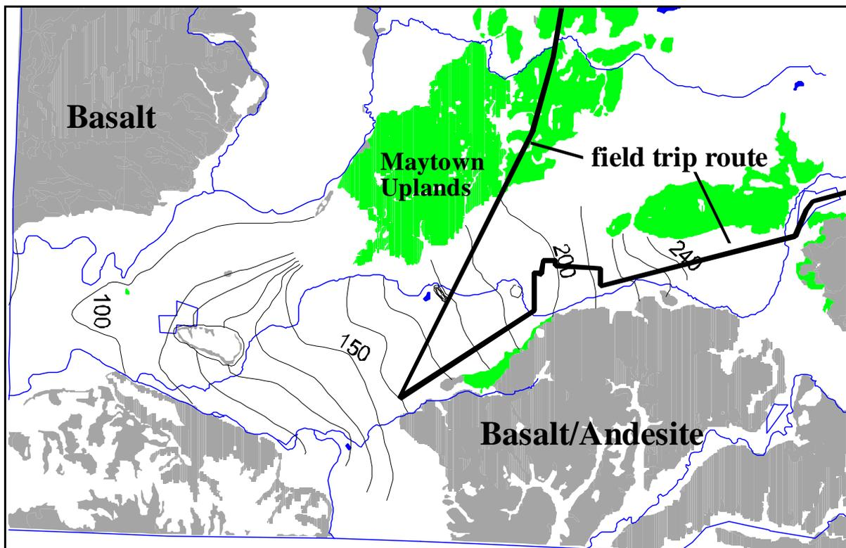
Groundwater in the Scatter Creek Aquifer generally flows from the east, near Tenino, to the west-southwest toward the Chehalis River, as described in Sinclair and Hirschey (1992). The lines shown in the figure on page 1 are contoured elevations of the hydraulic head measured in wells. The direction of groundwater flow is perpendicular to the contours in the direction of lower head. Flow directions change slightly throughout the year due to seasonal changes in recharge and discharge to streams.
